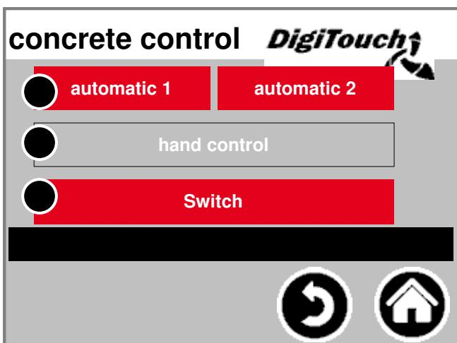
In this menu, you can Automatic and manual operation swap, and select. Of the selected mode is color deposited. Pressing the enters the currently selected mode one in the control of this mode. The mode can only be be changed if the Engine is stopped.
