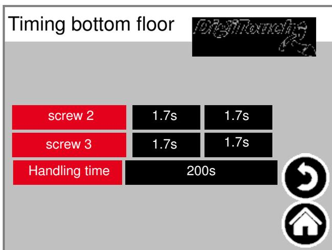
Desired pre- and post times the augers set to. To avoid unnecessary power consumption and tips any Substratverpressungen in the auger can avoid the turn of the individual Drive motors are temporally upstream and downstream. Enter the desired delivery time. The delivery time is the total duration of the forward and moving back Thrust wedge base in the supply air / dust channel.
